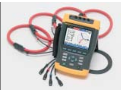
Fluke 435 with flex clamps
